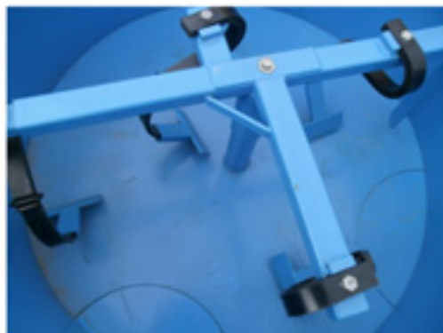
Cruciform arrangement of sprung stirring paddles and side scraper
