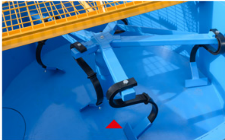
1.2 cubic meter version with pentaform stirring arm design
